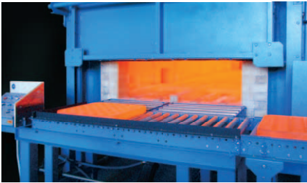
Internal chamber of 2-row pusher furnace with integral incineration
