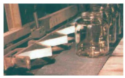
← REFRASIL heavy wall sleeving (HWS-1) covering assembly line equipment components provides protection against contamination and marking of hot glass containers.
